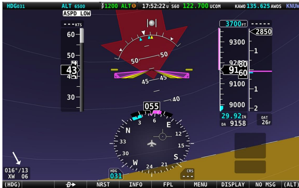
Figure 75 – Extreme Pitch Warning Indicator Arrows
