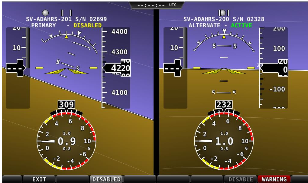
Figure 90 – ADAHRS Cross-Check Comparison (one ADAHRS disabled)
