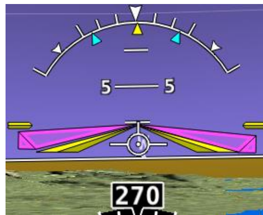
Figure 238 – Single Cue / Inverted-V with Autopilot Servos Not Engaged
