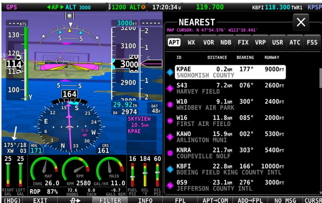
Figure 134 – Moving Map Nearest Window - FILTERED
