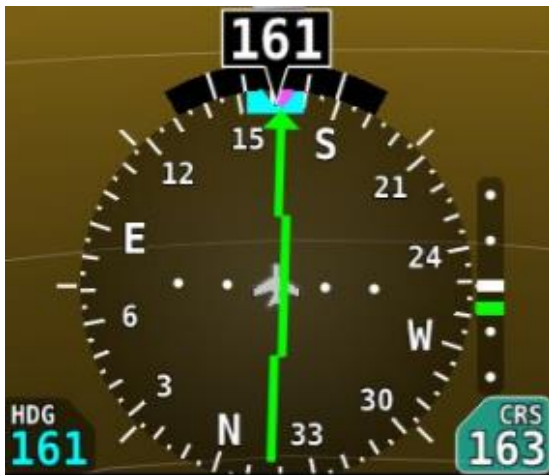
Figure 44 – HSI Example: Localizer
