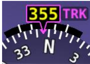
Figure 42 – GPS Track substitute for Magnetic Heading
