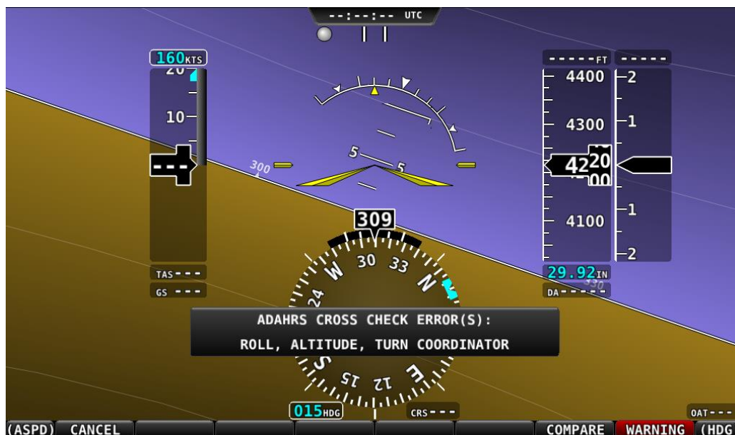
Figure 88 – ADAHRS Cross-Checking Disagreement
