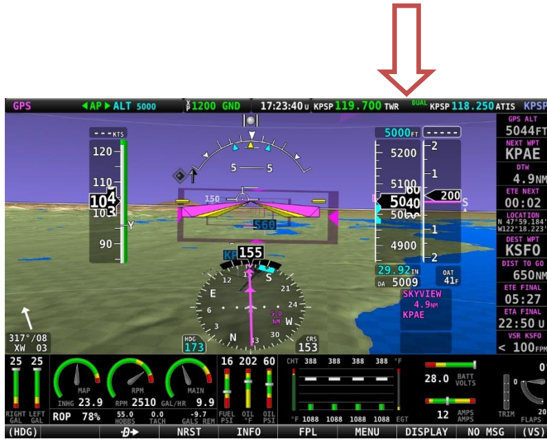
Figure 246 – SkyView Top Bar Com Radio Status Overview
