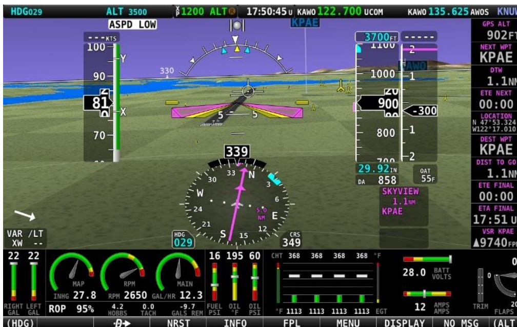
Figure 69 – SkyView HDX Synthetic Vision With Runways
