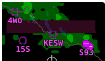
Figure 186 – Missing NEXRAD Data Blocks
