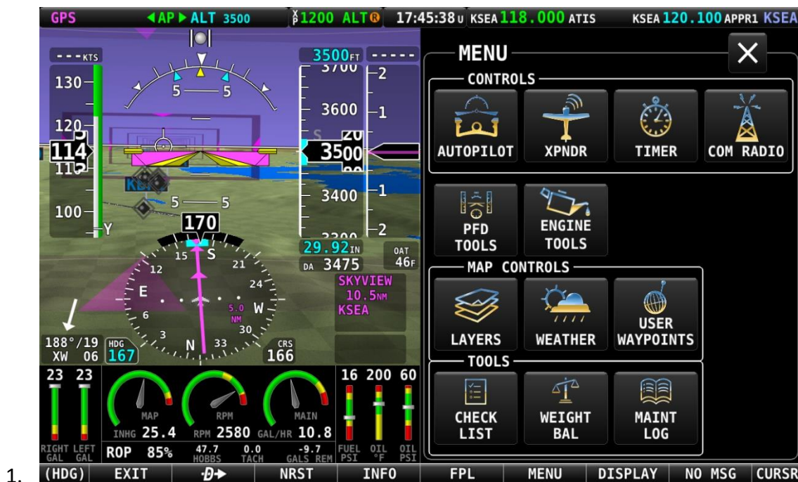
Figure 17 – ENGINE BOTTOM BAND partial over-written by MENU page
