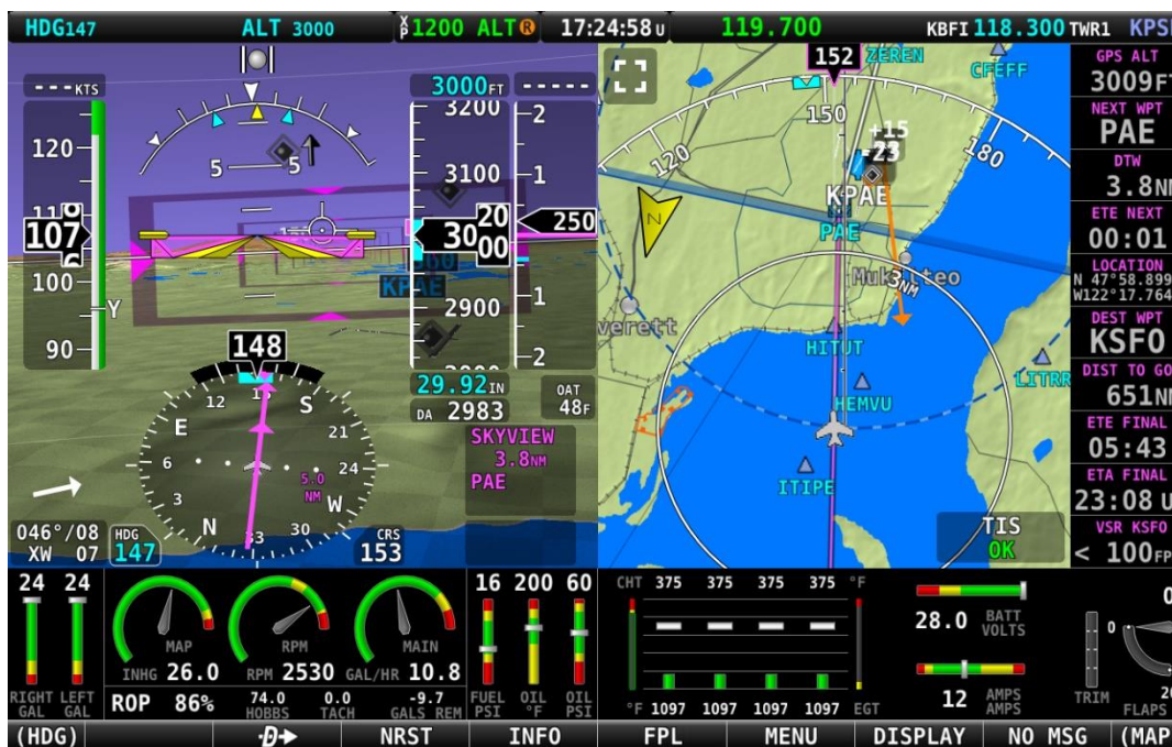
Figure 168 – Active Flight Plan: HSI and MAP Depictions
