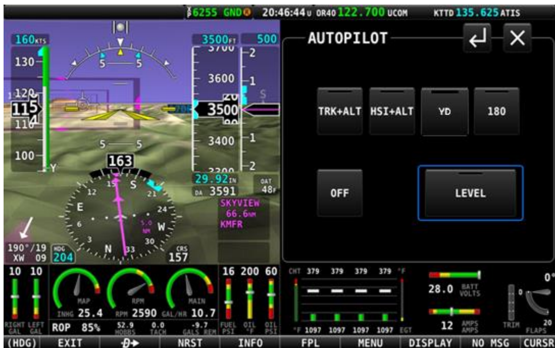
Figure 228 – AUTOPILOT Control page – Simplified Control Scheme
