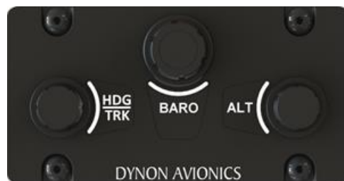
Figure 86 – SV-KNOB-PANEL – Horizontal version
