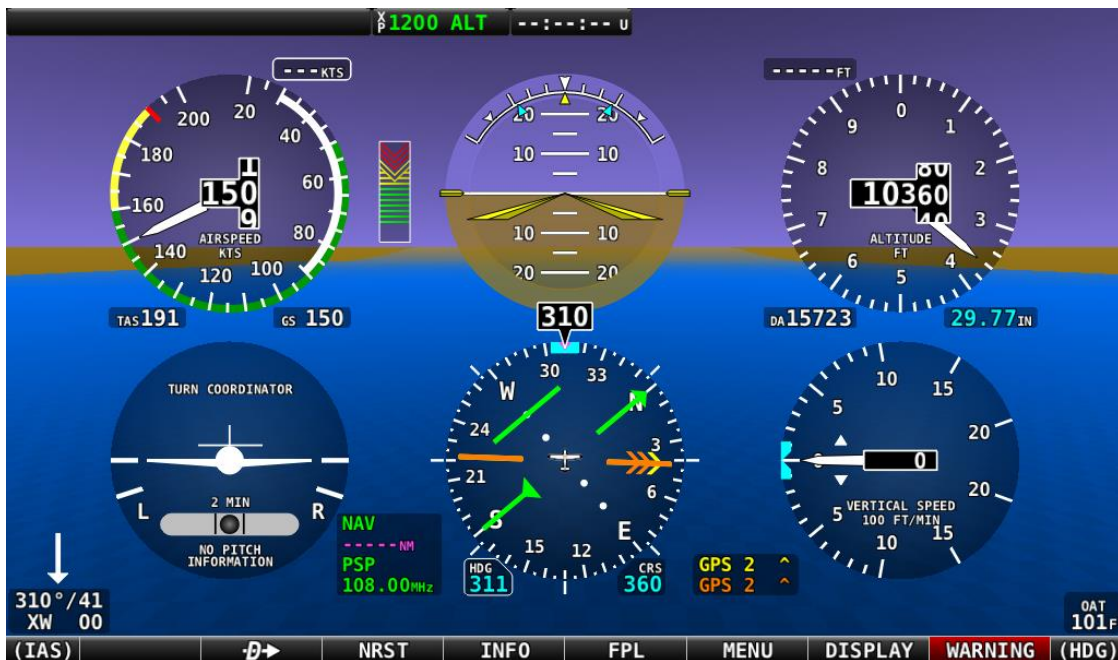
Figure 77 – Six Pack PFD Presentation, Synthetic Vision Enabled
