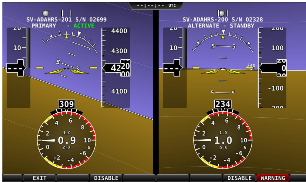
Figure 89 – ADAHRS Cross-Check Comparison (EFIS Presentation)
