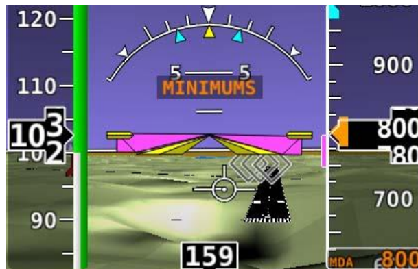
Figure 38 – MIN Bug and “MINIMUMS” Alert
