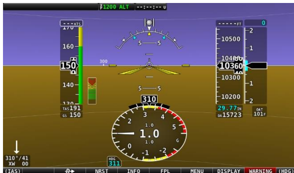
Figure 82 – G Meter in EFIS Presentation PFD
